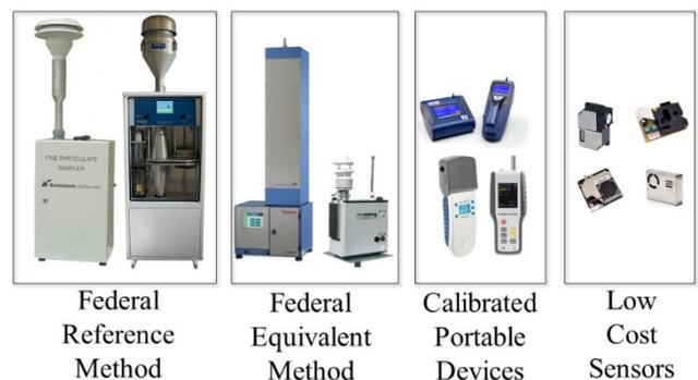
**Fig. 1.** Classification of PM measurement devices
