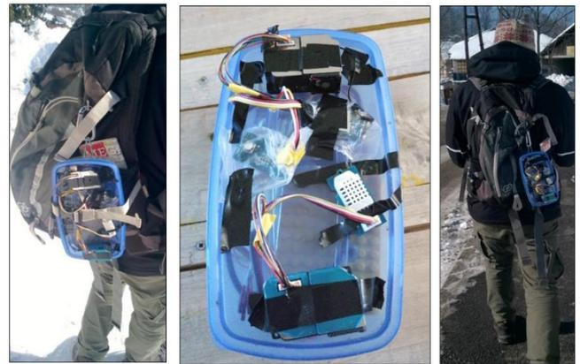
**Fig. 3.** The assembled measuring box and its position during the measurements
